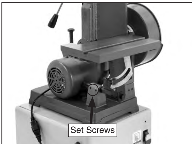
Figure 55. Location for removing work table assembly.
